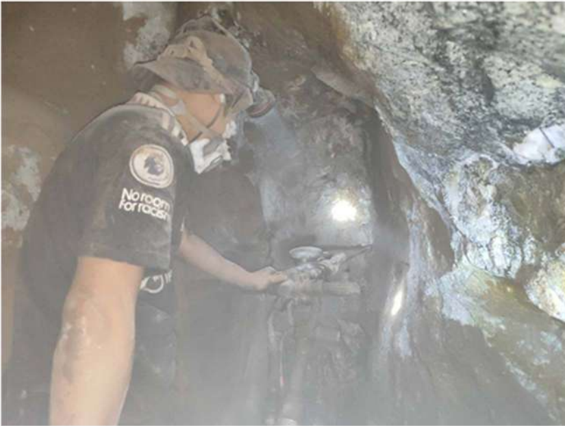
Figure 22 A drill operator holds an air gun, piercing the bedrock in the pit of Mawchi mine
