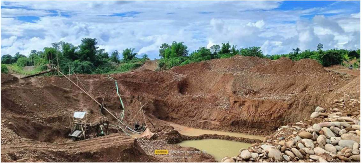
Figure 20 Gold mining operations employing the hydraulic mining method are taking place in Thar Yar Kaung village, showcasing a powerful technique where water is used to dislodge and transport gold-bearing material.
